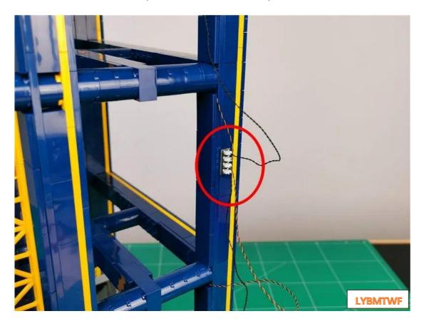
Organize the wires and properly twist the 30cm connecting wires
