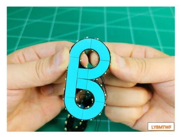
Go to the back of the letter and attach the wire between the light strips
