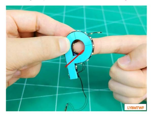
Attach the light strip to the middle of the letter P (wires facing down)
