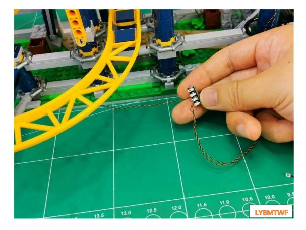
Insert the wires into the 4 sockets
