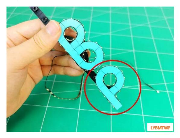
Tear off the back glue of the last section of the light strip, ready to be pasted to the letter L
