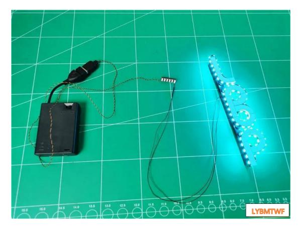
After the test, turn off the power, pull out the light strip, and leave the socket on the power supply
