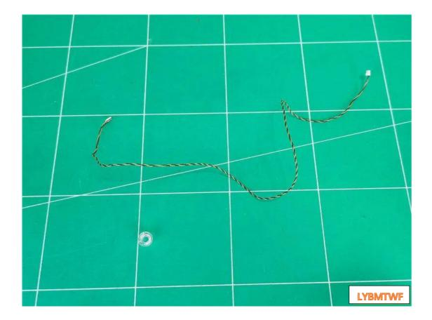
Pass the plug through the hollow hole
