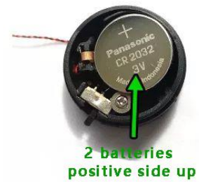
Button battery box (round) battery correct installation
