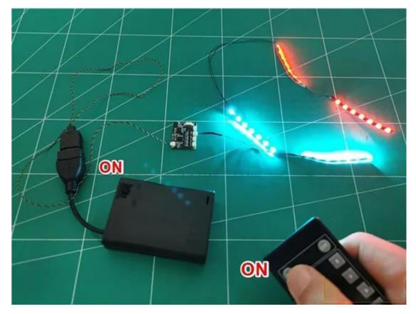
remote control ON button, and test that the light lights up normally
