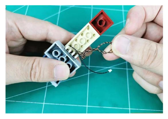
Screw the pellet wires together appropriately
