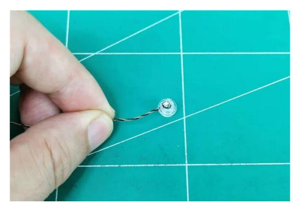
Attach the light-emitting side of the lamp to the side of the hollow round hole
