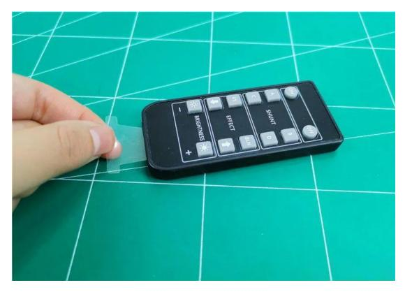
Remove the remote control and pull out the lower insulation spacer
