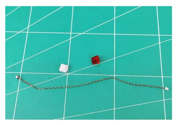
Bond the light-emitting side of the lamp to the gray bump with the wires facing either side
