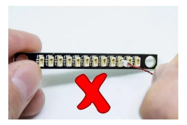
When installing light pellets on building blocks, make sure they are placed correctly (yellow LED components exposed). You can place them directly on top of the building block studs or in between.
