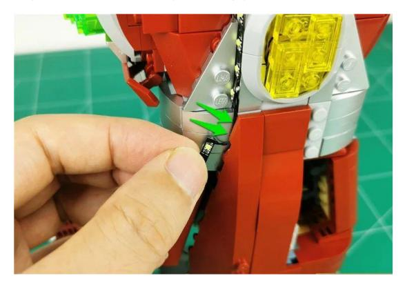
Plug the wires between the strips into the gap shown
