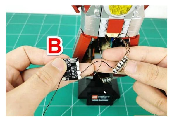
Insert the cable on the 6-seat into the module B socket
