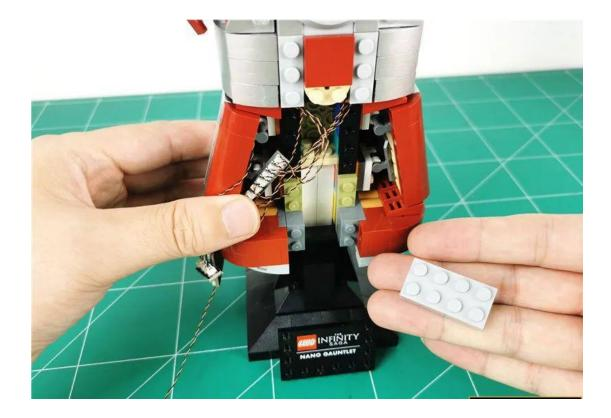
Attach the light grain wire to the center of the circle
