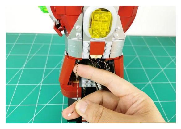
Insert the thumb lamp plug into the remote control module A socket (marked near the socket).
