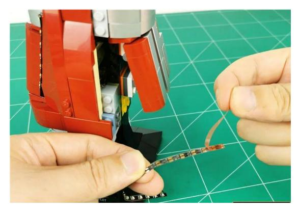
Peel off the adhesive backing of the light strip on the head
