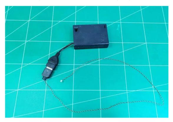
Remove the USB power cable and insert it into the battery compartment
