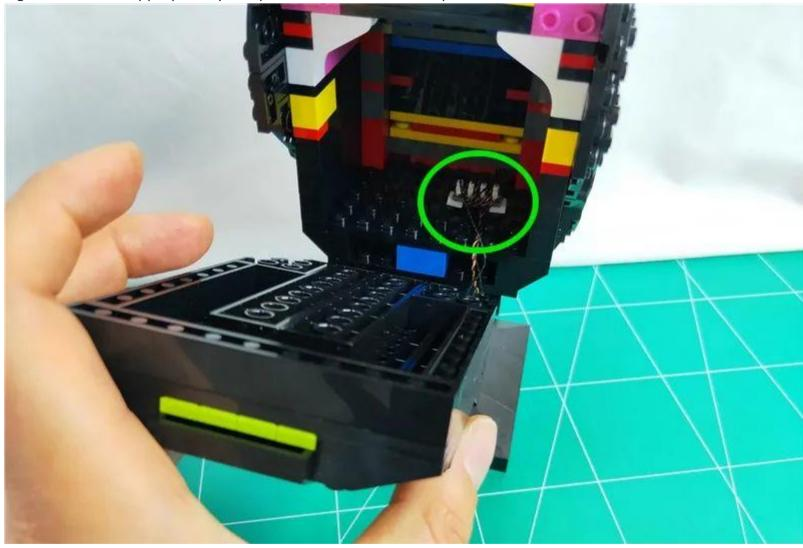
Tighten the wires appropriately and paste the 4 seats into the position shown
