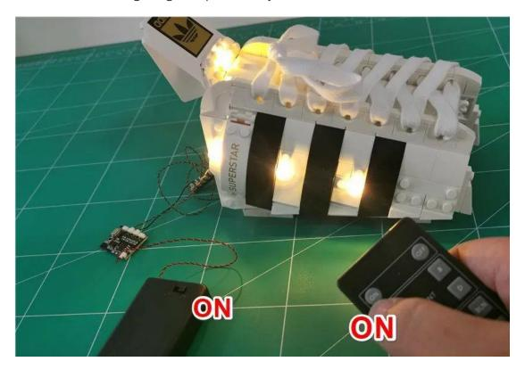
After the test, click the remote control OFF to turn off the power and temporarily stuff the remote control module and battery box into the shoe
