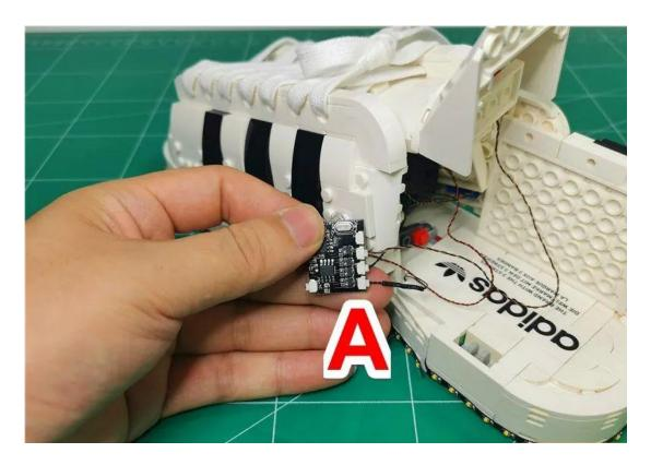
Insert the heel light into the remote control module D socket
