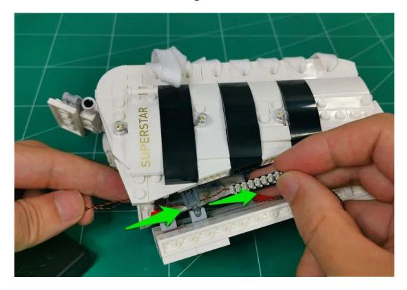
Insert the two plugs on the far right into the 8-seater
