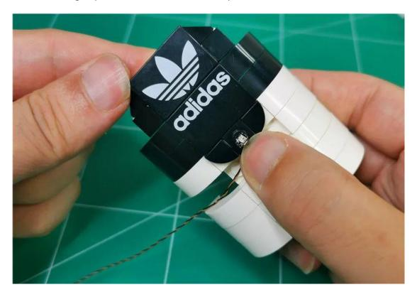
Secure the lamp particles with a transparent circle
