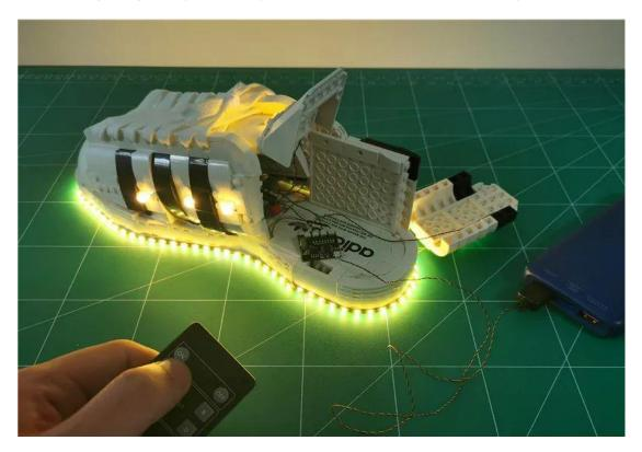
Tuck the module into the shoe and remove the white part indicated by the arrow
