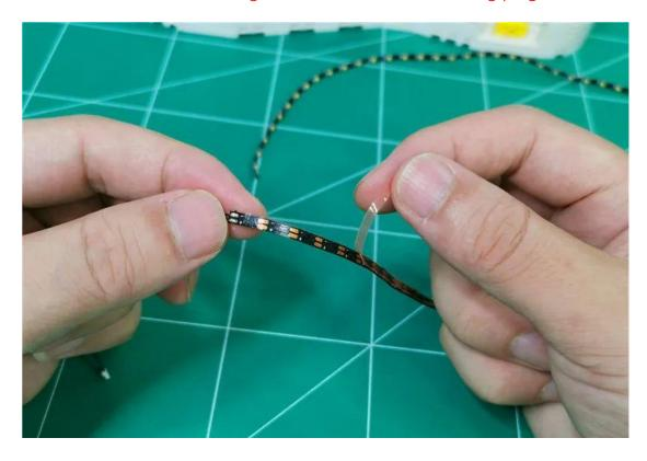
Attach the light strip to the bottom edge of the sole and paste it to the place shown
