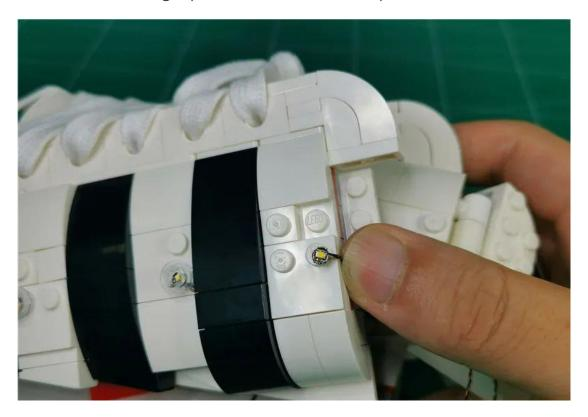
Fix the lamp particles with a transparent circle and pass the wire through the angle
