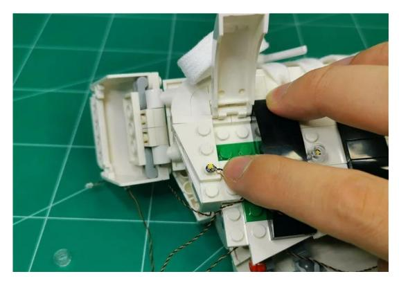
Fix the lamp particles with a transparent circle and put 2 wires together and pass along the angle
