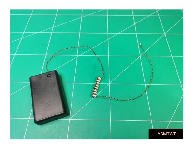
Turn on the battery compartment switch and test that the light lights up normally
