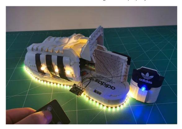
After the test, turn off the power and tuck the module into the shoe
