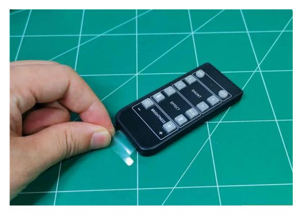
Turn on the battery compartment switch, click the remote control ON button, and test that the light lights up normally
