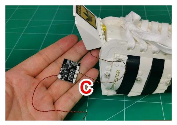
Insert the 5cm cable on the 8 seats into the module B socket
